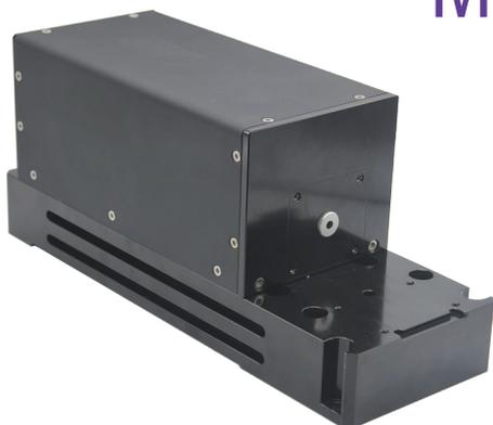
RealLight's MCO series energy adjustable sub-nanosecond microchip laser with free space output, is composed of integrated electronic control module for energy adjustment, photodetector module and laser drive board. This laser features compact design, plug and play, and free space output with a beam divergence lower than 2mrad.
