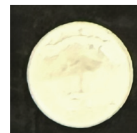
Beam profile (2940nm)
